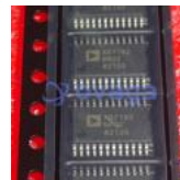
AD7192BRUZ-REEL Analog Devices, Inc TSSOP-24
